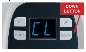
Once the door has reached the desired open position, press 'SET' to save in the units memory and 'CL' (Close) will show on the display. Press and hold the 'DOWN' button until the door reaches the desired closed position and press 'SET' to save in the units memory.
