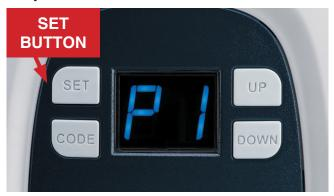
Starting with the door in the closed position, press and hold the 'SET' button until 'P1' is visable on the display
